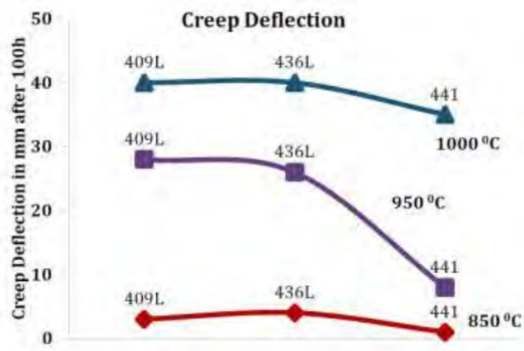
Figure 5: Creep Deflection at different temperatures.
