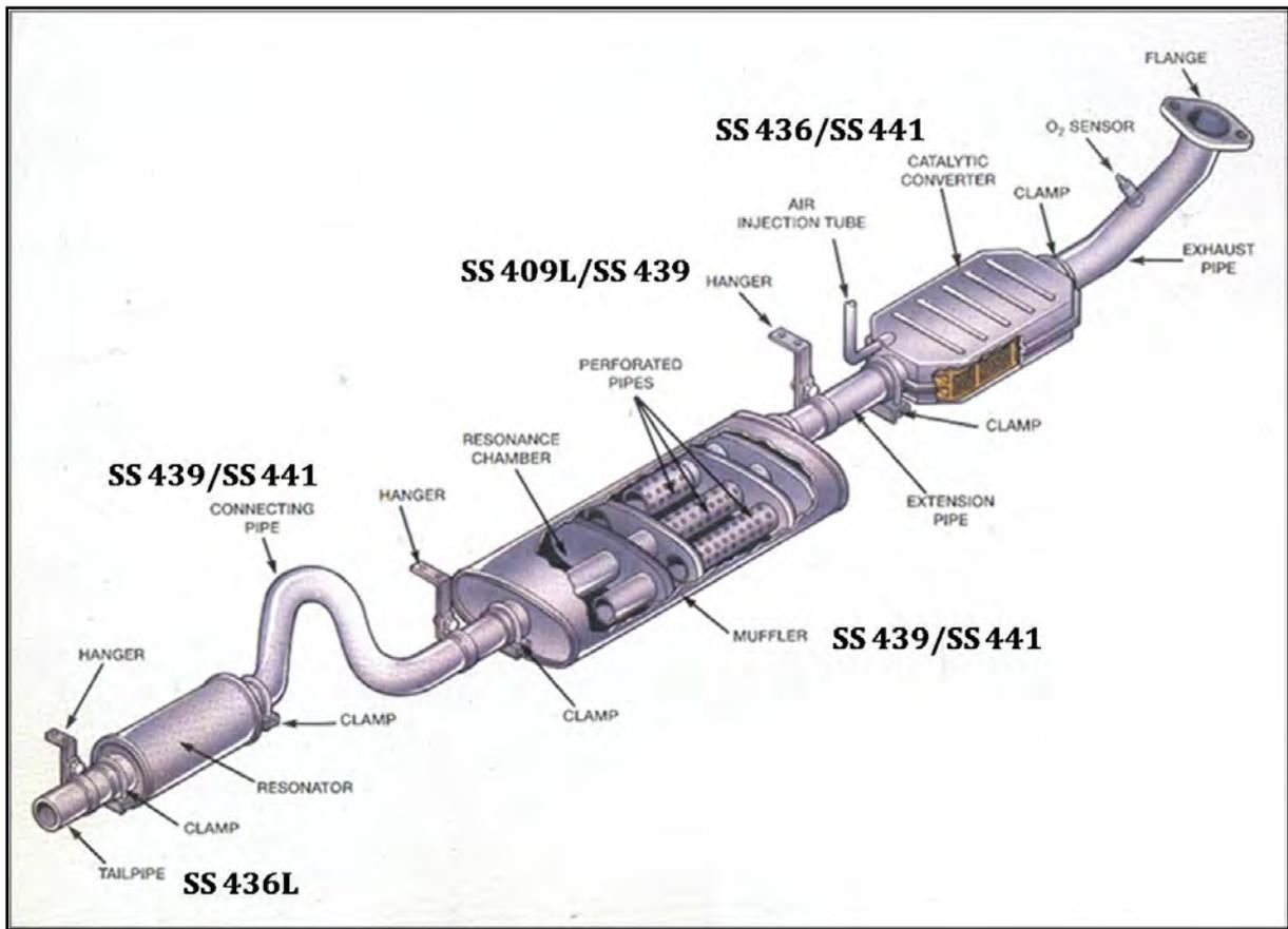
Figure 2: Automotive Exhaust System
