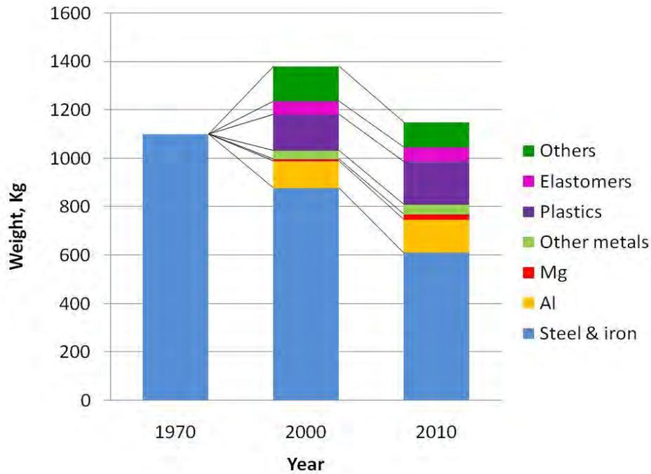
**Figure 1: Materials used for manufacturing cars**
