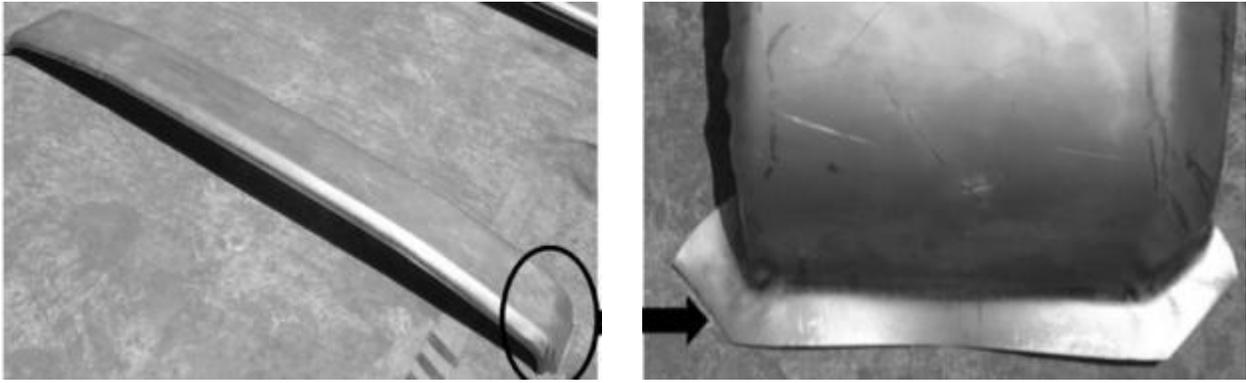
**Figure 6: Bumper made of JSLT**
