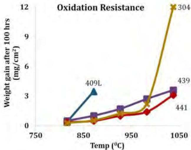
Figure 3: Weight gain in 100 Hrs of Oxidation in still air at elevated temperatures
